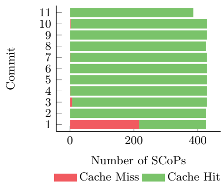
FIGURE 6.2: Cache hits and misses for each commit with default settings and no generalization
