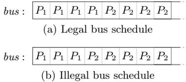
Figure 8: Bus schedule with bus-processor ratio 4
